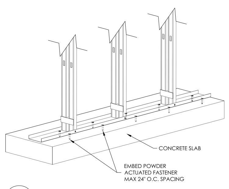
SG-2 Sound Guard Base-of-Wall Anchor Detail
